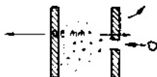
Fig. 11. Impact of a particle, about 0.5 mm in size at a velocity of approx. 10 km/s on the double wall as indicated below, decomposed into many droplets upon penetrating the first wall (lower photograph), the droplet cloud impacting on the second wall with some droplets piercing the wall (upper photograph).
